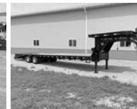
'18 PJ 35, 1-owner, 30' w/5' beavertail, 102" wide, low pro, hyd. jacks, tdm. dually, torque tube, monster ramps, 12,000# axles, disc brakes, oil bath hubs, never seen salt, very nice, removable top deck, $27,500.
